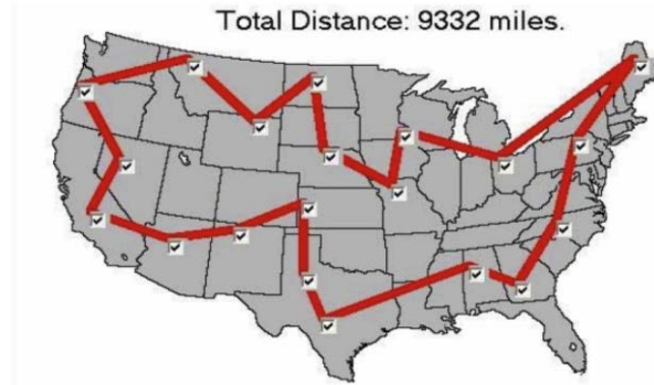
Figure 1: The TSP Solution for a 20-City Problem Having 6.1 \times 10^{16} Permutations (from: http://www.solver.com/solver-platform-sdk-source-code-examples.html )
