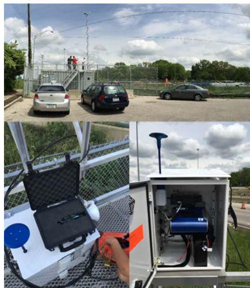
Figure 2: Portable Monitors Used for Air Pollution and Noise Measurements
