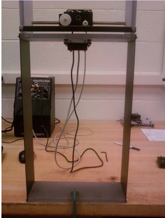
Figure 15. Single storey, with active mass damper.
