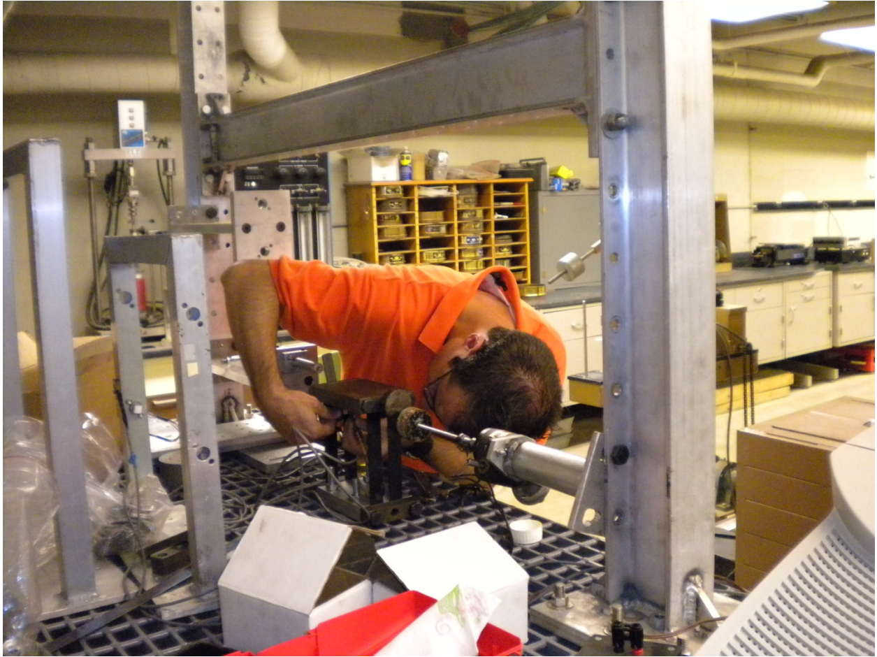
Grant installing the viscous damping device.
