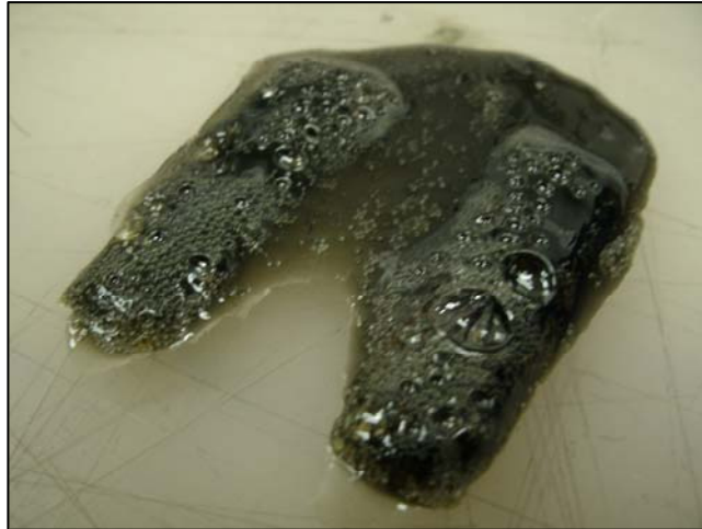
Figure 14: Toolfusion sample; note: this sample contained a large number of bubbles and was not suitable for testing
