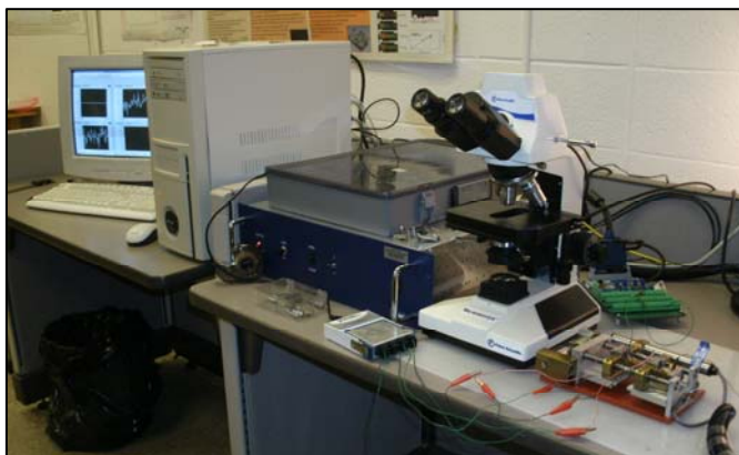
Figure 7: Apparatus for analyzing stress and resistance in bending load for composite sample
