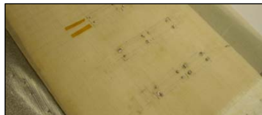
Figure 4. CNT threads bonded to Teflon fabric using conductive epoxy
