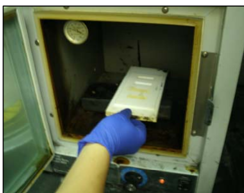
Figure 22: Heat cured composite samples are removed from molds, planed and conductive wire leads are attached with conductive
