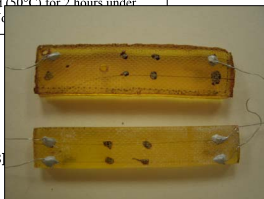
Figure 22: Heat cured composite samples are removed from molds, planed and conductive wire leads are attached with conductive
